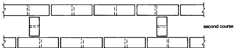
Alternative bonding using quoin blocks
